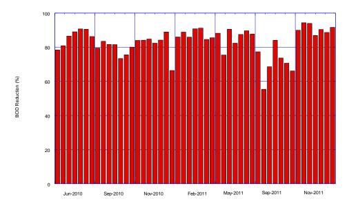
In addition to the removal of contaminants of organic pollution, the treated wastewater discharged from the BTF also contains low concentrations of ammoniacal nitrogen (typically less than 3 mg/L) resulting in a reduction of approximately 50 percent in terms of total nitrogen. The BTF also achieves a reduction in indicator bacteria (i.e. faecal coliforms and enterococci) of between 99% to 99.5% during normal operation of the BTF.
