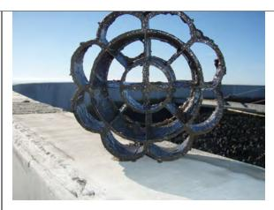
View of a Plastic Media (Petal) piece showing biomass growth (with 1 – 2mm covering) – taken from the full scale Biological Trickling Filter Plant
