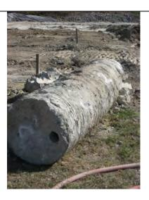
A deep soil mix column is removed and core for testing as part of the ground strengthening work, February 2008
