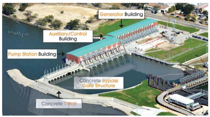
Figure 1: Aerial photograph of the 17th Street station with major PCCP components labeled. Interim control structures, which are now being removed, are visible in the lower right hand of this photograph. All three stations were designed for the water hydrostatic, boat impact, wave, 200-mph hurricane wind, and unbalanced loads resulting from the stability analysis for each structure.
